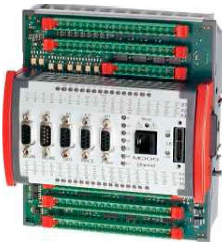
Figure 2. The Moog Servo Controller PLC
